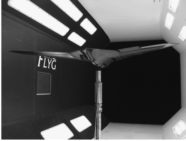
Fig. 1 Yaw setup in the low-speed wind tunnel.
